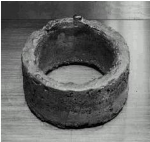
This ring is almost 100% pure plutonium. At just 11cm in diameter and weighing 5.3kg, it is enough for one modern nuclear bomb core. (Photo: Nuclear Archive)
